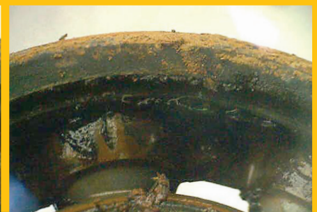
COMPETITIVE BEARING (B) AFTER 200 HOURS OF USE
