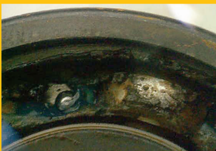
TORO BEARING AFTER 200 HOURS OF USE
